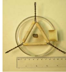
Figures 1a and 1b. Preparation of Burnt Bloodstains: glass microscope slides with bloodstain smears were suspended face-down over a 10 cm diameter glass Petri dish filled with 10 ml of absolute ethanol for the burn experiment.
