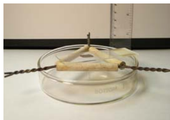
Figures 1a and 1b. Preparation of Burnt Bloodstains: glass microscope slides with bloodstain smears were suspended face-down over a 10 cm diameter glass Petri dish filled with 10 ml of absolute ethanol for the burn experiment.
